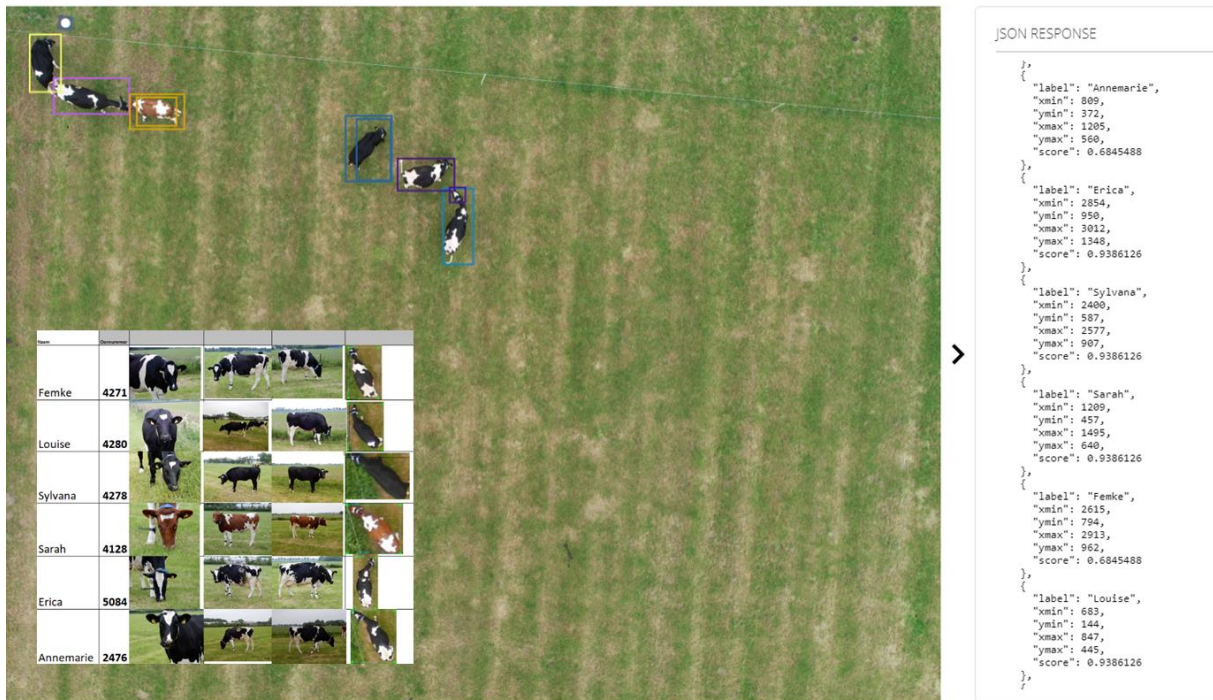
Figure 1 Individual cow identification at CARUS, the research facility of the Department of Animal Sciences, part of Wageningen University, using a Phantom 4 at 40 meter height. The experiment in May 2019 included 6 Holstein Frisian cows with different fur patterns.
